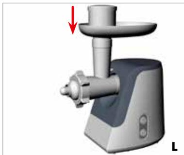
**IMPORTANT:** If the tools overlap the edges of the worm housing the worm is not placed properly inside of the worm housing. Turn the worm a little
